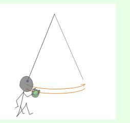
• Swing the pendulum remembering to respect the condition of small oscillations (oscillation amplitude less than about 1/10 of the pendulum length *L*).
