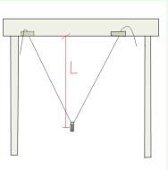
• The oscillating mass will naturally move into a symmetrical position with respect to the two suspension points. However, we recommend a quick visual check before using the pendulum for measuring activities.
