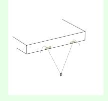
• **Caution!**. The pendulum length L will be the distance between the center of gravity of the suspended mass (the center of the nut) and the lower edge of the support.
