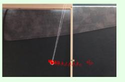
• As body position is tracked, Tracker offers both the *x*(*t*) graph of the horizontal component of the position and the numeric data (see columns below). [Working in conditions of small oscillations we will neglect the deviations of the oscillating mass from the x direction.]
